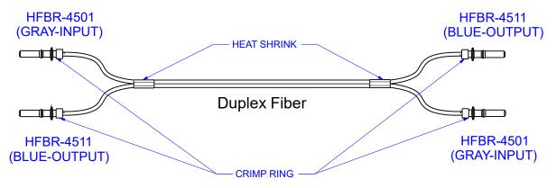
\*The fiber cable used for the assembly will be based upon the category of cable used for the SERIES. Asahi Kasei and Mitsubishi Eska optical fiber cable are shown, however other manufacturers' cable may be used based on availability.
