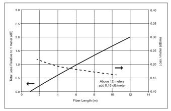
FIGURE 4. Fiber Loss in GH4001
