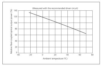
FIGURE 2. Optical power output versus temperature  $(I_F=20mA)$
