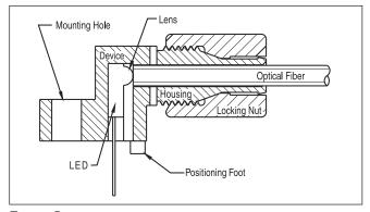
FIGURE 5. Cross-section of fiber optic device.
