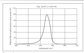
FIGURE 1. Relative intensity versus wavelength.
