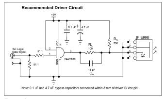
FIGURE 3. Typical interface circuit. (IF = 35mA).
