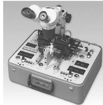
*Photo 20. Fusion splice for glass optical fiber.*
