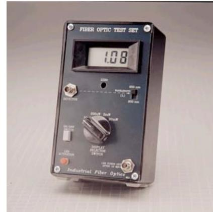
*Photo 21. Optical power meter with a built-in light source.*
