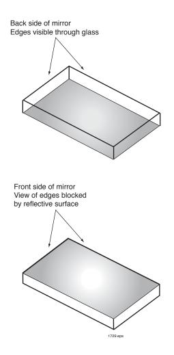
Figure 6. Identifying the "first surface" side of a mirror.
