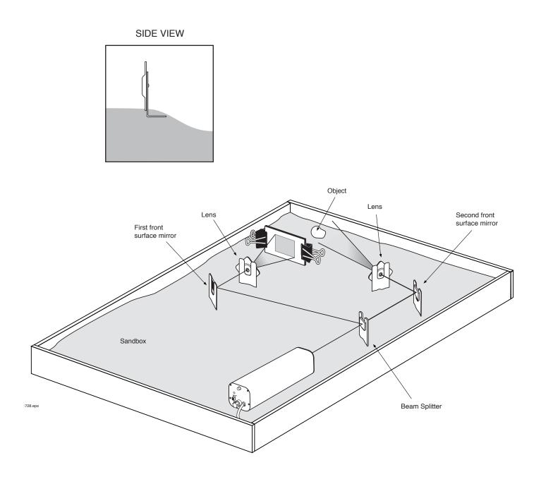
Figure 4. Typical holography setup in the sandbox.
