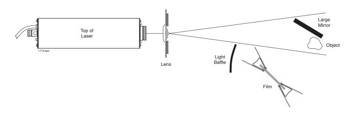
Figure 18. Setup for capturing a one mirror transmission hologram.
