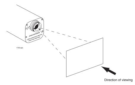
Figure 14. Viewing a transmission hologram.
