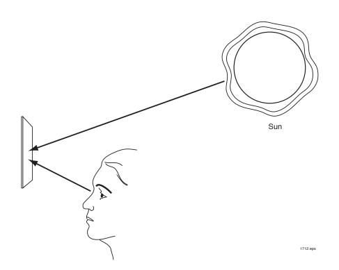
Figure 13. Viewing a reflection hologram.
