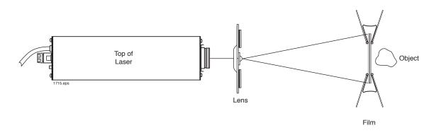
Figure 16. Setup for capturing a direct beam reflection hologram.
