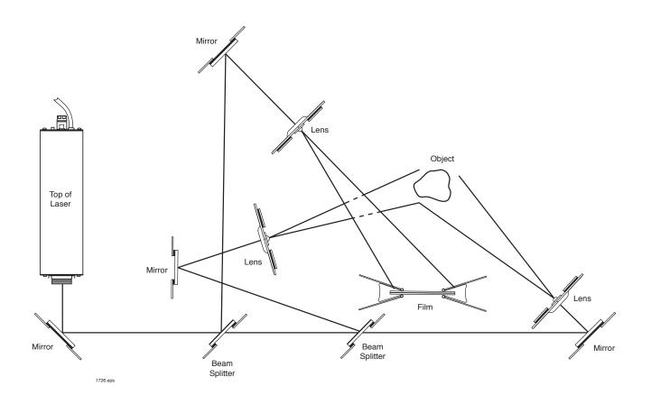
Figure 25. Setup for capturing a hologram using multiple lighting sources.
