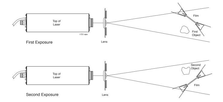
Figure 27. Setup for capturing a multiple channel transmission hologram.
