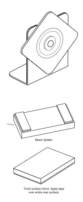
Figure 2. Using magnetic tape to mount the optics.
