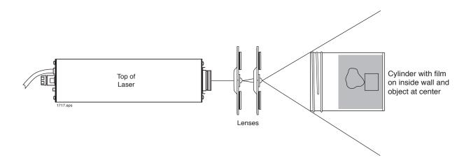
Figure 19. Setup for capturing a 360° transmission hologram.
