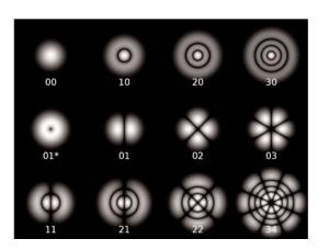
Figure 5a. Examples of Transverse Electromagnetic Modes (TEM<sub>pl</sub>).
