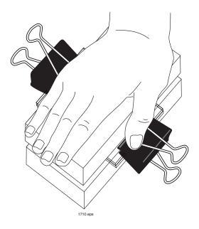
Figure 11. Squeezing out air bubbles.
