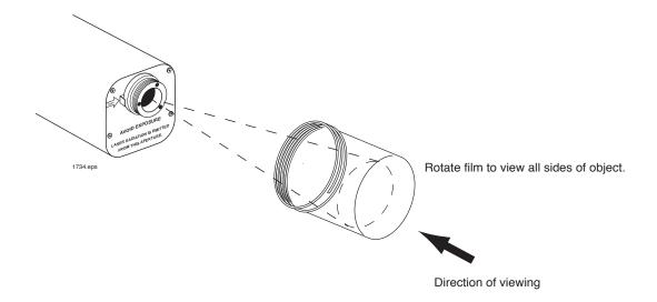
Figure 15. Viewing a 360° hologram.
