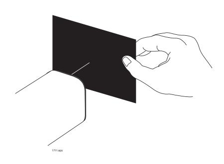
Figure 12. Shutter card raised just before film exposure.
