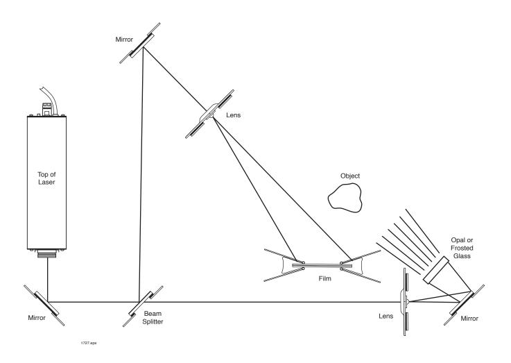
Figure 26. Setup for capturing a hologram using soft lighting techniques.
