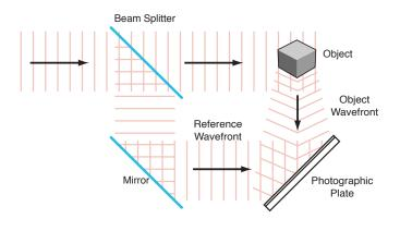
Figure 1a. Recording a hologram.
