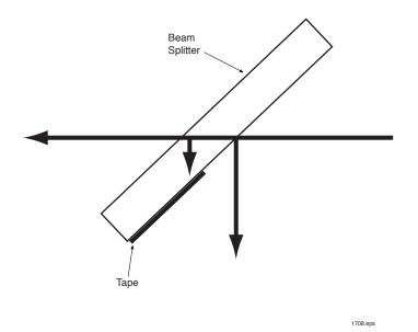
Figure 7. Blocking internal reflections inside the beam splitter.
