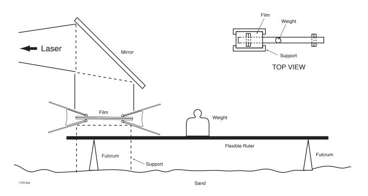
Figure 28. Setup for double exposure holometry.
