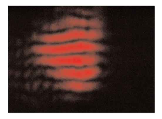
Figure 9. Interference fringes produced by the Michelson's Interferometer.
