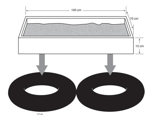
Figure 3. Completed sandbox with innertubes.
