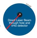
Figure 4. Close up view of the alignment laser beam to receiver aperture.
