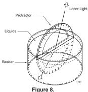
Refraction of a laser beam.
