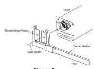
Figure 6. Variable slit diffraction.
