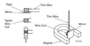
Figure 5. Construction of an optical Galvanometer.
